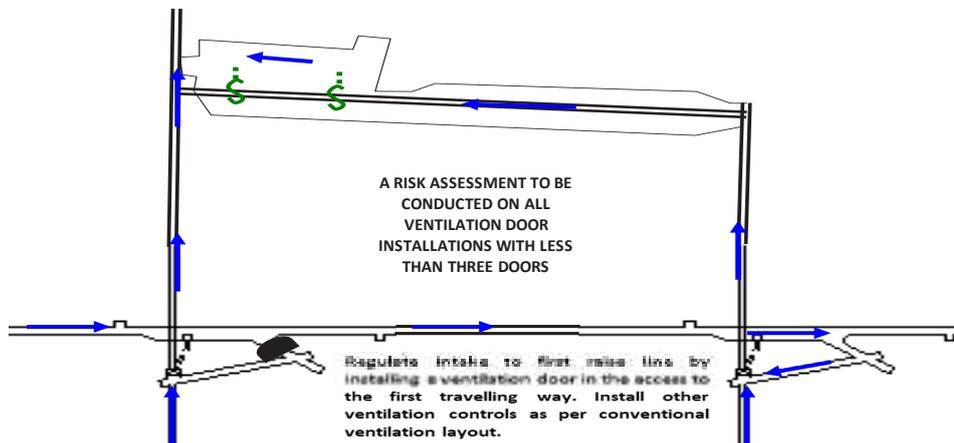
Install ventilation door set in drive between raise lines and regulate air distribution with a brattice set to ventilate the **u-tube**. Management of water control is critical.
