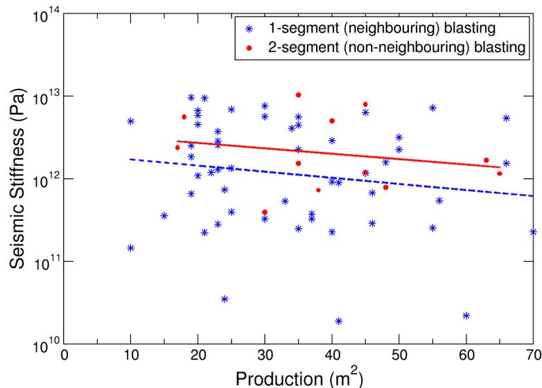
Figure: Seismic Stiffness resulting from different kinds of production.
