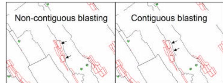
Figure: An example of a contiguous (right) and non-contiguous panel blast at Mponeng
