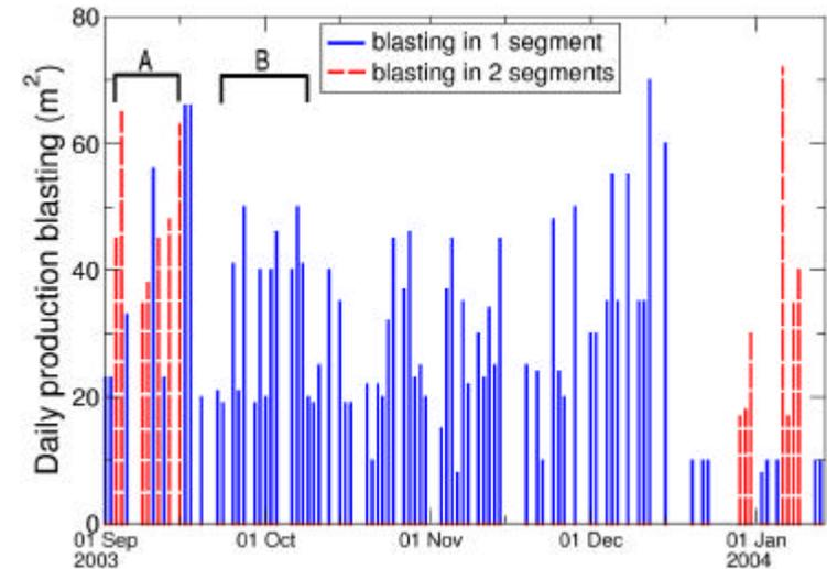
Figure: Amounts and types of blasting in the 104/109 48-49 pillar at Mponeng. During time “A” the blasting was mostly of type 2-segments, while during time “B” the blasting was only of type 1-segment.
