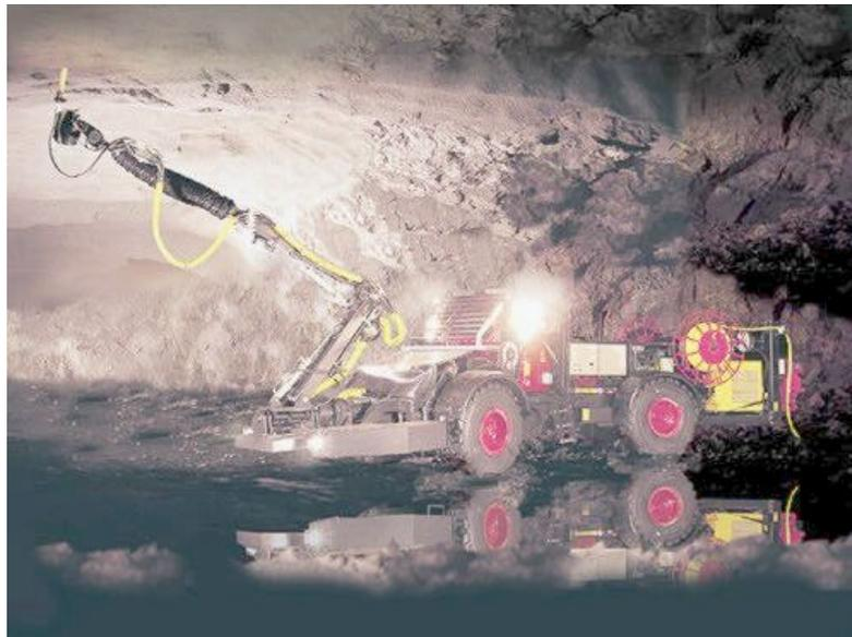
Figure 6-3 Mechanical scaling machines
