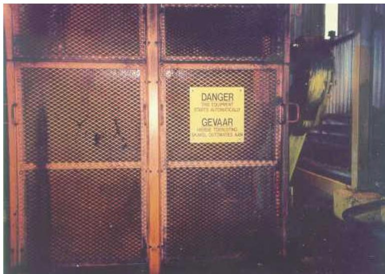
**Figure 4: Effective guarding around drive pulley**
