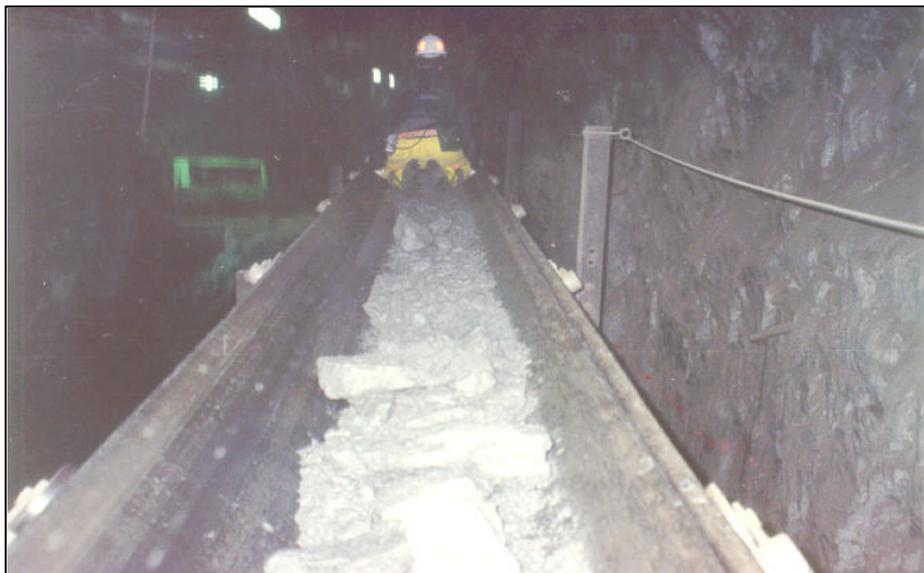
**Figure 7: Man riding with material on conveyor**
