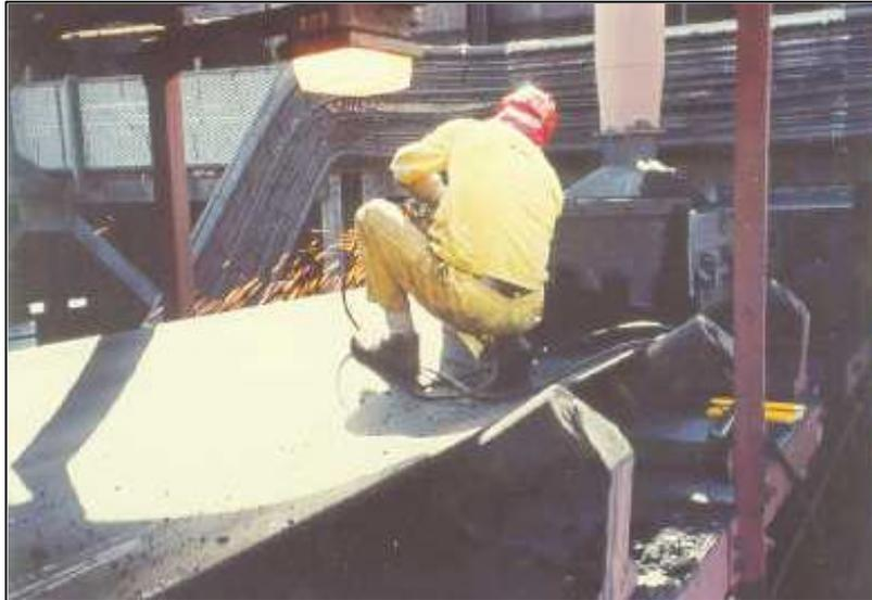
**Figure 3: Man on conveyor belt performing maintenance after locking out**
