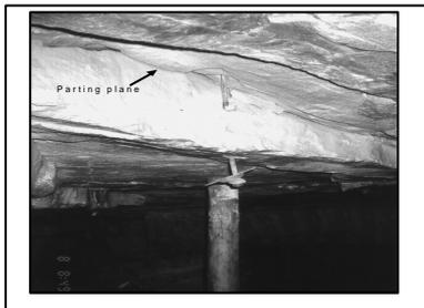
**Figure 1 Hangingwall layering suitable for rockbolting (Kinross Mine). Note bearing plate loosened during blast.**
