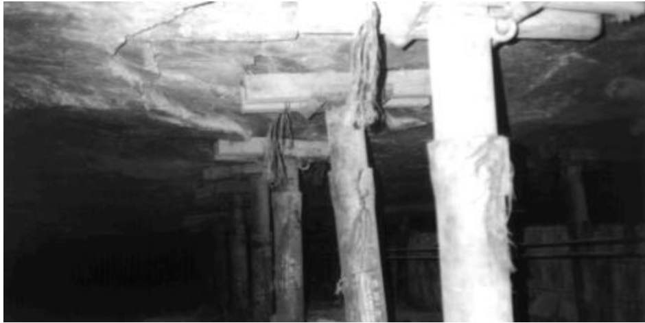
Figure 4.8.6 Example of a hangingwall with FPFs.
