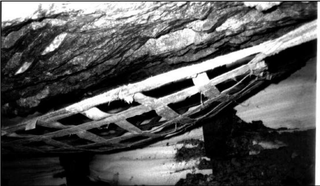
**Figure 3.7.18**      *Net showing signs of wear after seven blasts.*
