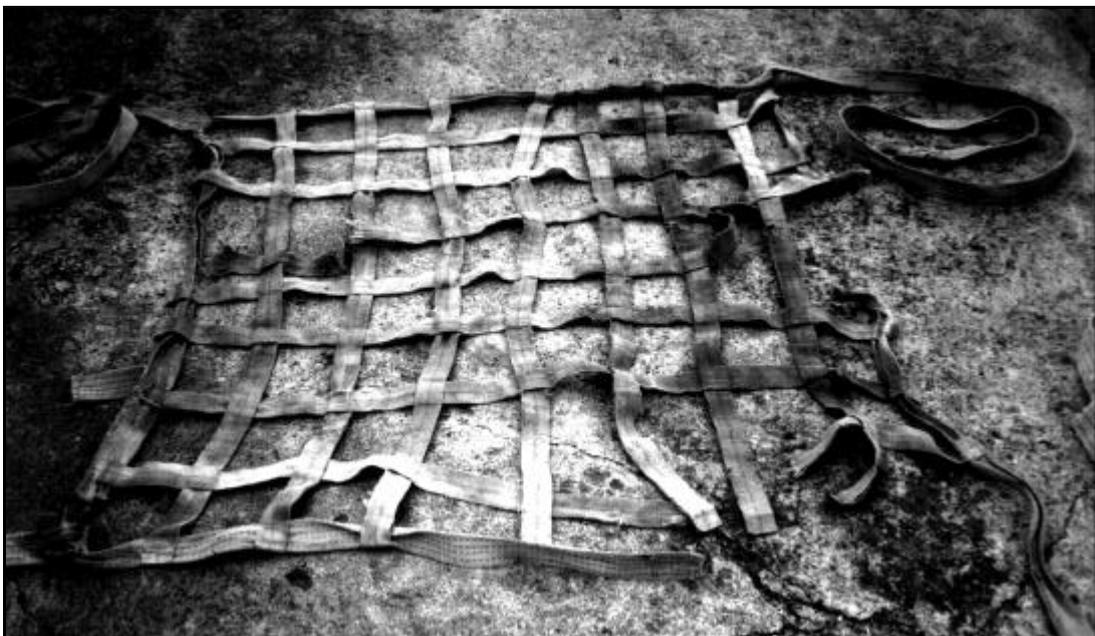
**Figure 3.7.20**      **Note perimeter webbing broken as a result of having been caught by the scraper.**
