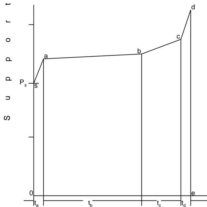
**Figure 3.7.8 Typical form of variations in support resistance (Peng et al., 1982).**
