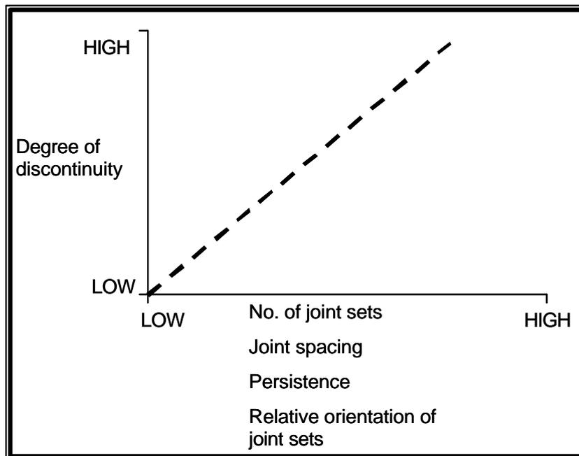
**Figure 3.3.6 Influence of joint characteristics on the degree of discontinuity.**
