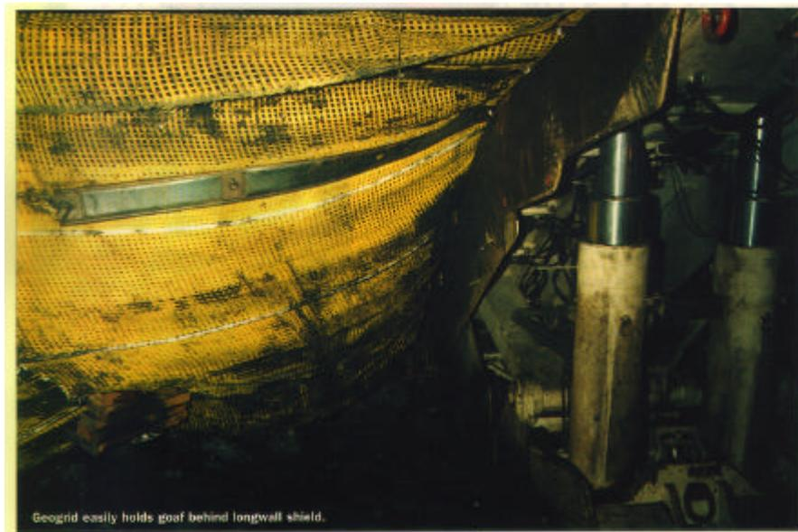
**Figure 3.7.21**      *The Geogrid easily holds the goaf behind the longwall.*
