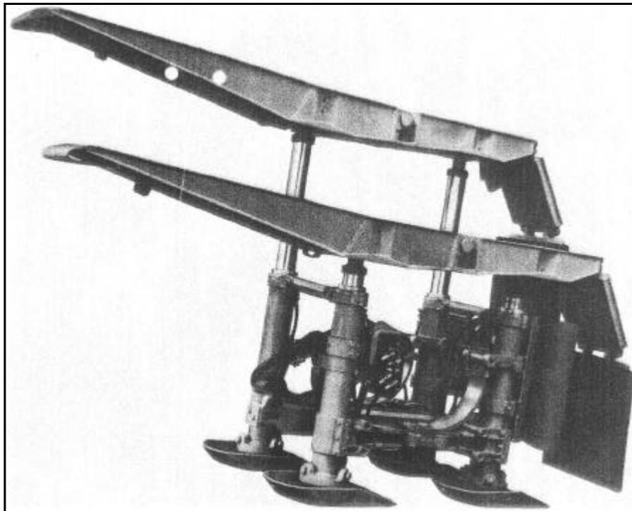
**Figure 3.7.3** *Layout of Frame support.*
