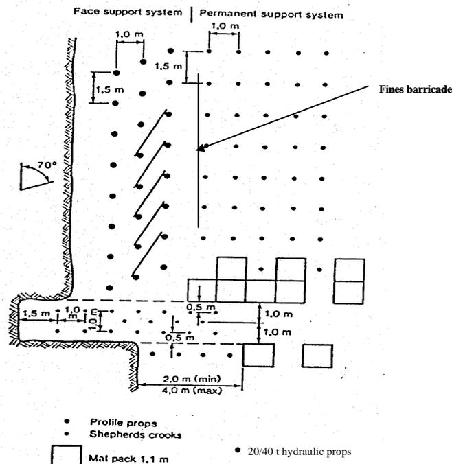
**Figure 3.7.24** 20/40 t blast-on face support system (after Glisson and Roberts, 1991).
