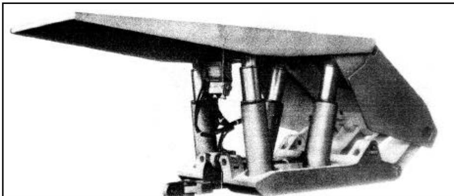
**Figure 3.7.6  $4V/600_{0.85}$  chock shield.**
