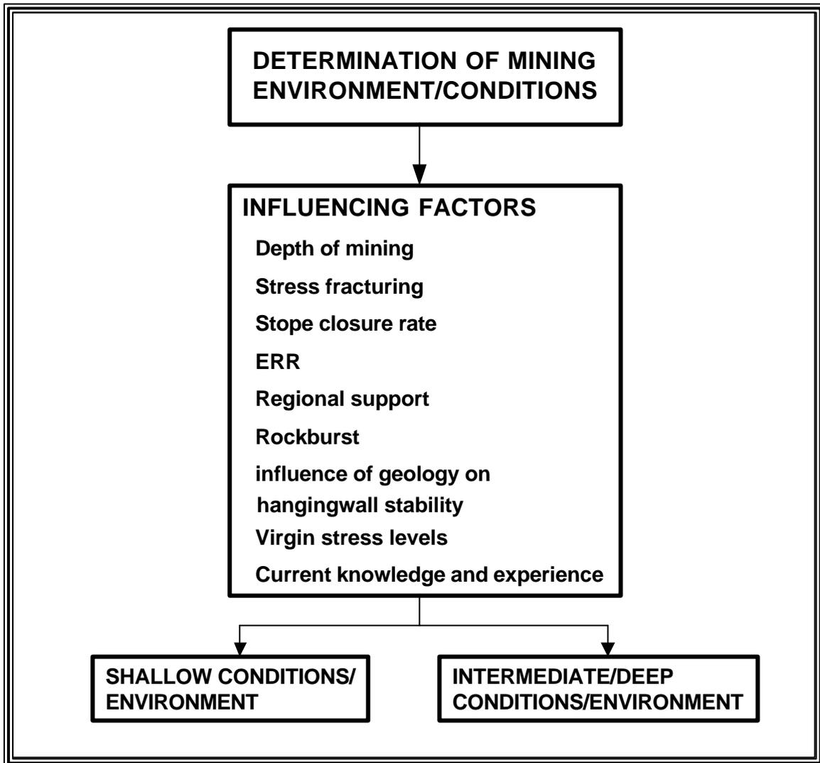
*Figure 3.2.1 Flowchart determining mining environments and conditions.*
