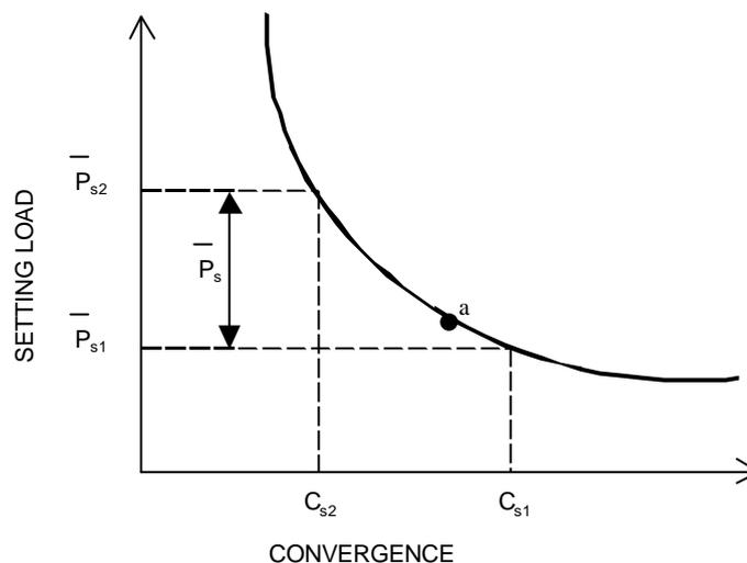
**Figure 3.7.7 Setting load versus roof convergence.**
