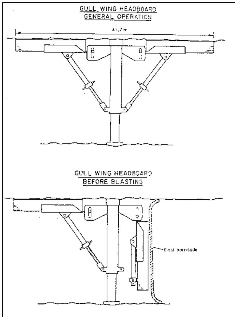
**Figure 3.7.13 Gully wing headboard in general operation and just before blasting (after Spearing, 1992).**
