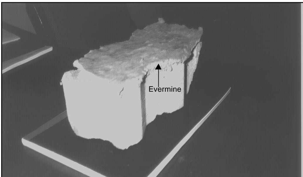
**Figure 3.7.9 Photo showing cured Evermine on brick after dynamic load test.**
