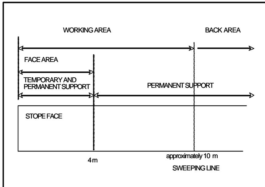
**Figure 3.1.1** Diagram illustrating the face area.
