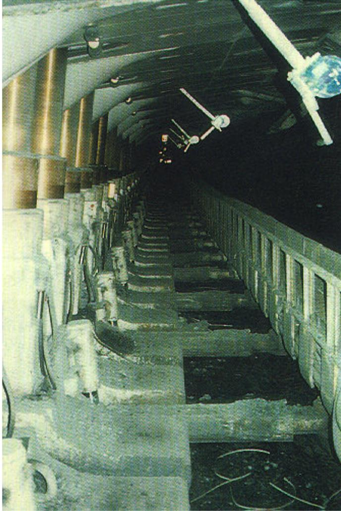
**Figure 3.7.23 View along longwall showing the boat winches; every second support positioning the mesh roll tightly against the canopies.**
